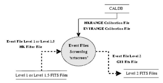
Figure 4.5: The flow diagram for the Stage 2 processing all modes
