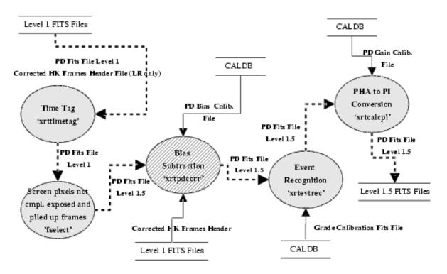
Figure 4.3: The flow diagram for the Stage 1 processing of the Photodiode mode
