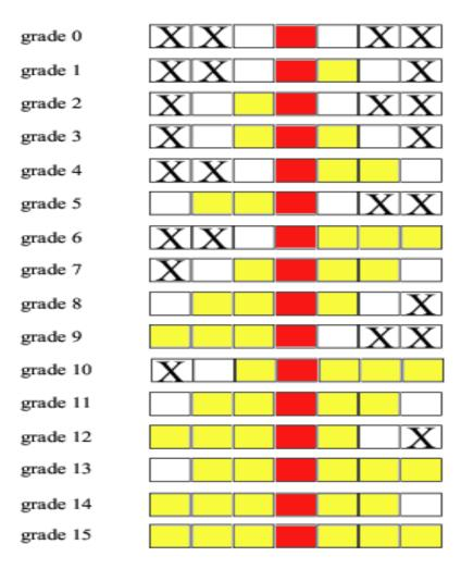
Figure 2.3: The definition of the XRT grades for Timing modes
