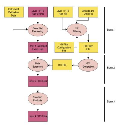
Figure 4.1: The flow diagram of the XRTDAS pipeline
